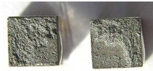
Fig. 4. The typical image of the TE pellet destruction.
