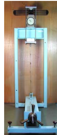
Fig. 3. Tensile machine for determination of Ni layer adhesion strength.
