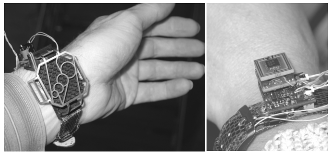
Figure 7. Wireless sensor for tracking the power produced on humans: the TEG (left) and electronic module (right). environmental conditions and TEG behavior at these different conditions. Fig. 7 shows the completed system.
